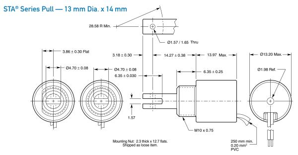
STA® Series Magnetic Latching Pull — 13 mm Dia. x 16 mm
