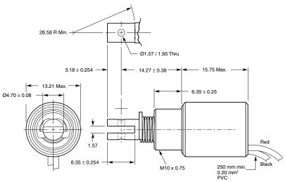
STA® Series Push — 13 mm Dia. x 14 mm
