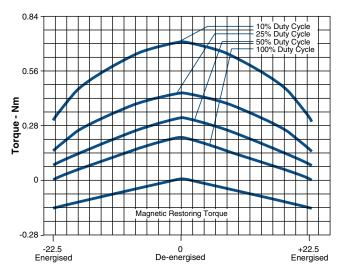
Graph 1 shows three position operation. In any mode, the armature seeks centre of stroke at zero power. Applying a positive or negative voltage causes the shaft to rotate clockwise or counter clockwise. When power is removed, the restoring torque is applied to the load, or alternatively, the shaft can be driven to centre under power.
